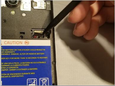
Disconnect the battery connector flex cable by sliding the black spudger under the wires and carefully prying up the entire terminal casing.
