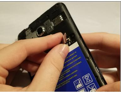
Remove the metal bracket covering the battery connector flex cable. Now that it's unscrewed, it should come out easily.
