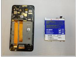
Remove the blue battery by lifting it straight up, or by gently turning the phone over into your palm and catching the battery as it comes out.
