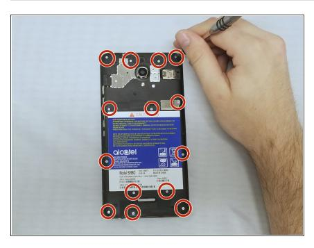
Using a Phillips #000 screwdriver, remove the fourteen 3mm screws that connect the housing and the battery.
