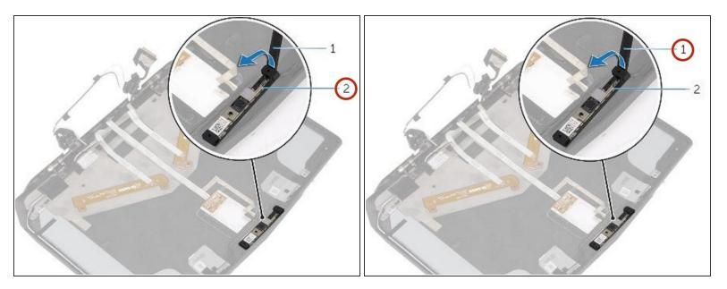
Using a plastic scribe, pry the camera module off the display back-cover.
