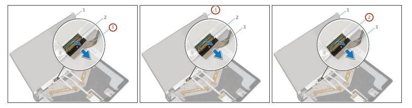
Connect the display cable to the NEW display panel and press down on the connector latch to secure the cable.
