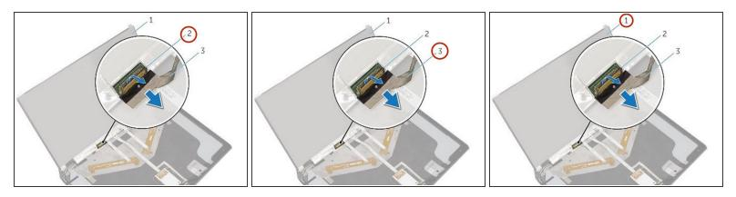
• Lift the connector latch and disconnect the display cable from the display panel.
