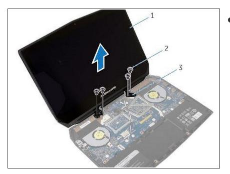
Align the screw holes on the hinge caps with the screw holes on the display hinges.
