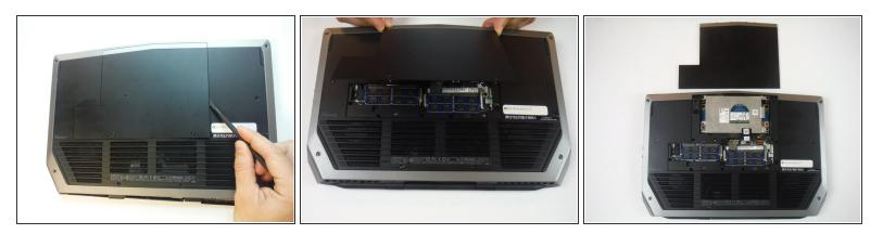
• Remove the small access panel using a heavy duty spudger.
