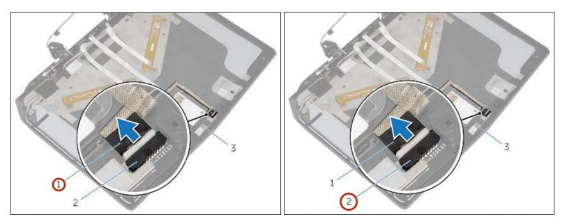
• Disconnect the camera cable from the camera module.
