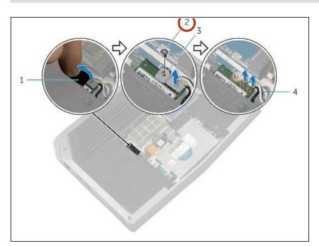
• Remove the screw that secures the wireless-card bracket to the wireless card.
