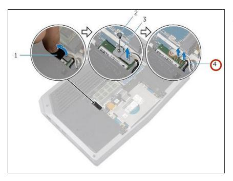
• Disconnect the antenna cables from the wireless card.
