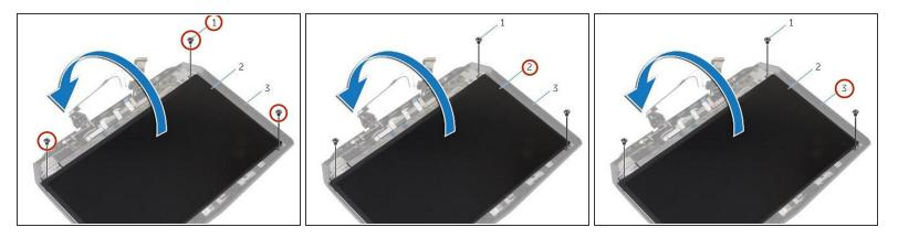
• Remove the screws that secure the display panel to the display back-cover.
