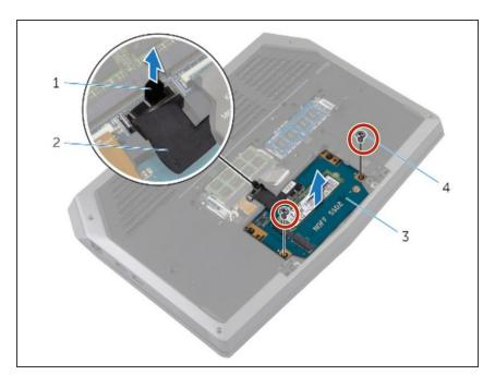
Align the screw holes on the solidstate drive assembly with the screw holes on the computer base.
