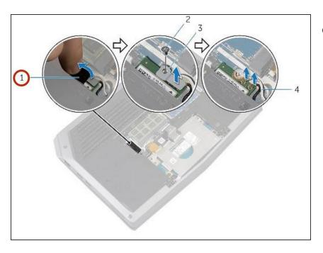
• Peel off the adhesive tape from the wireless card.
