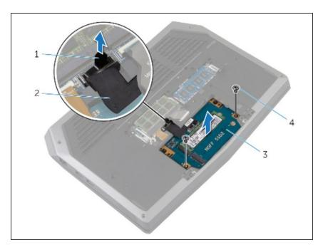
Replace the screws that secure the solid-state drive bracket to the solidstate drive assembly.
