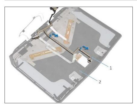
Note the display cable routing and peel the camera cable off the display back-cover.
