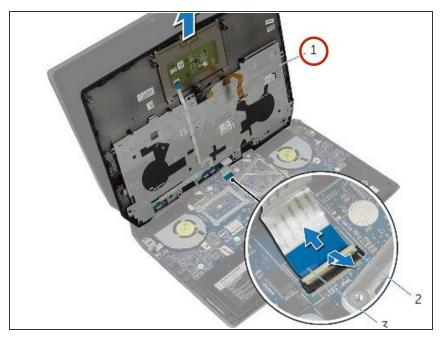
Align the palm-rest assembly on the computer base and snap it into place.
