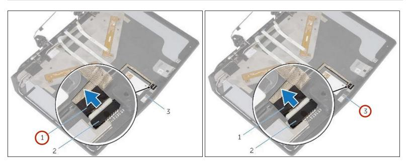
• Connect the camera cable to the camera module.
