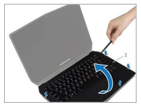
Using a plastic scribe, pry up along the edges of the palm-rest assembly.
