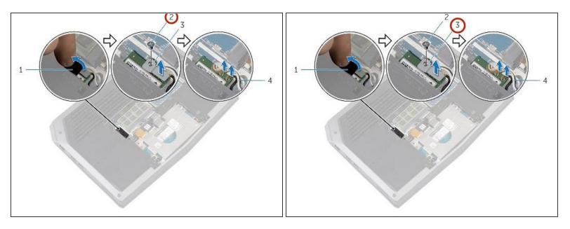
• Replace the screw that secures the wireless-card bracket to the wireless card.
