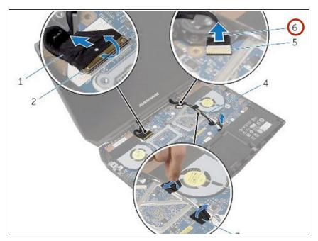
• Route the logo-board cable through the routing guides on the display hinge and connect the logo-board cable to the system board.
