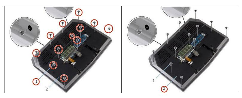
• Remove the screws that secure the palm-rest assembly to the computer base.
