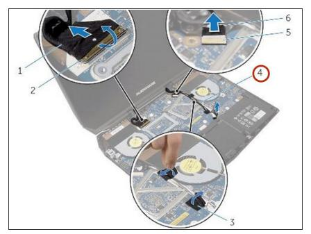
• Remove the antenna cables from the routing guides on the display hinges.
