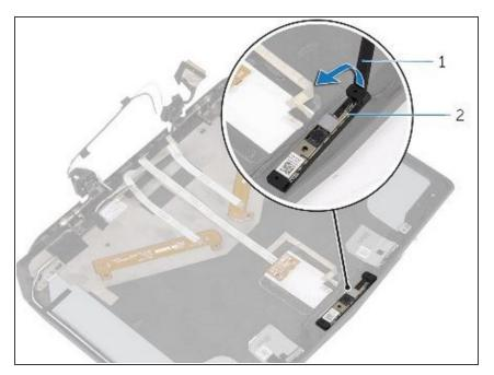
• Using the alignment posts place the **NEW** camera module on the display back-cover and snap it into place.
