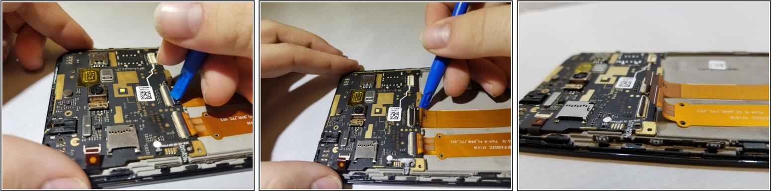
**i** When disconnecting the ribbon cables from the clamps, do not peel the cables up. They're glued down.
