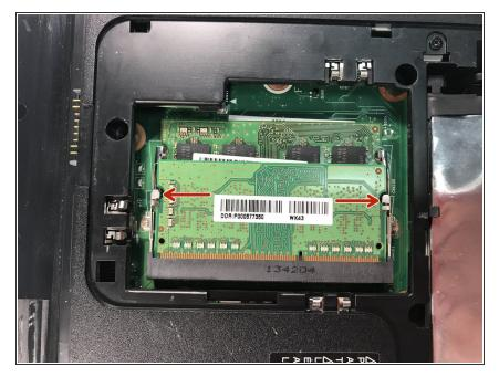
Once the ram chip is exposed, push the two clips away from the ram chip to release it. (Clips move in direction of arrows.)
