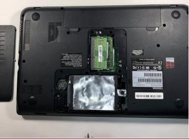
Using your Phillips #1 screwdriver, unscrew the 6mm screw on the panel, exposing the hard drive and RAM.
