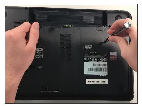
On the back of the laptop, remove the 6mm Phillips #1 screw. This screw is attached to the keyboard.
