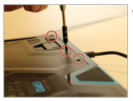
Turn over the keyboard and remove the three screws using a Phillips #0 screwdriver.
