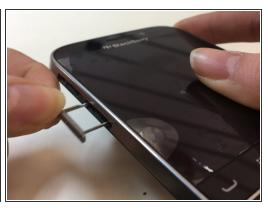
Use a SIM tool to remove the SIM and micro SD card trays.
