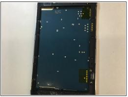
Be sure to add adhesive to the new battery, and replace the foam on the connector.
