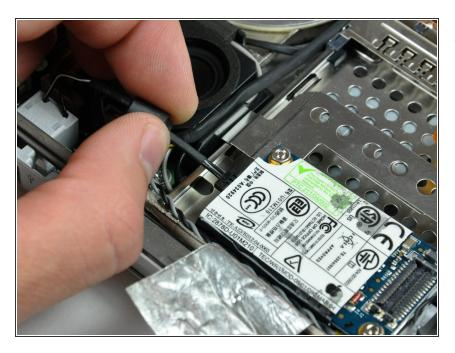
Disconnect the RJ-11 cable from the modem.
