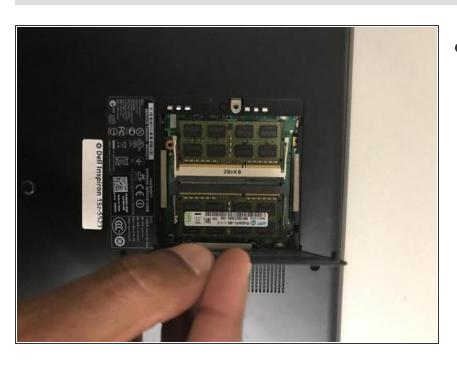
Remove the back-plate from the computer by grabbing it and pulling up.
