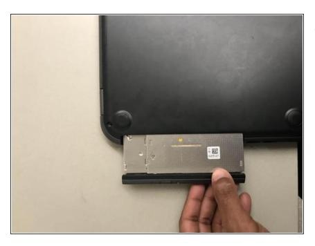
Once the Back-Plate is off use your fingers to grab onto the CD Reader and pull straight out.
