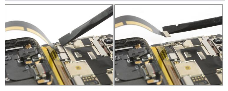
• Use a spudger to pry up and disconnect the charging port and headphone jack flex cable.
