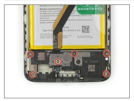
• Remove the six Phillips #00 screws (2.9 mm length).
