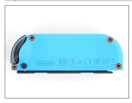
Use a Tri-point Y00 driver to remove the four 6.3 mm-long screws from the back panel of the Joy-Con.
