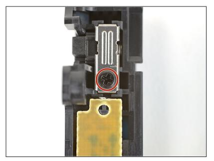
Use a Phillips #00 driver to remove the screw securing the buckle lock retaining bracket.
