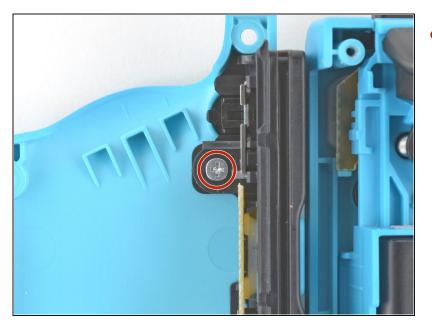
Use a Phillips #00 driver to remove the 2.5 mm screw securing the charging rail.
