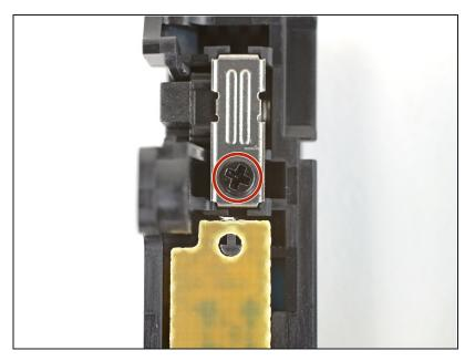
Use a Phillips #00 driver to remove the screw securing the buckle lock retaining bracket.
