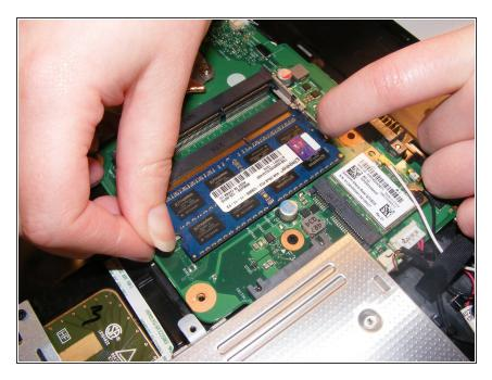
• Using your fingers, unclip the two side clips.
