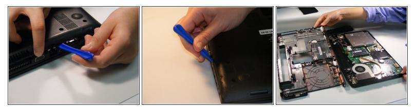
• Using the plastic opening tool, remove the outer panel and set to the side.
