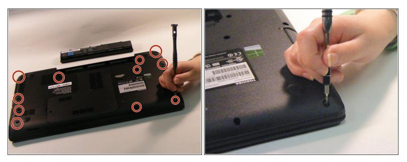
• Using the Phillips #1 screwdriver, remove the eleven 2.5mm screws.
