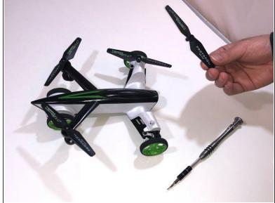
Hold the propellers gently and pull the propellers out of the drone.
