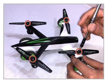
Using a Phillips #0 screwdriver, remove the four screws connecting the propellers to the device.
