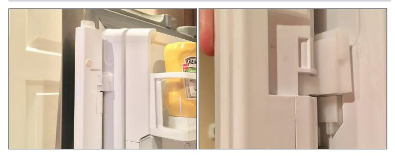
• Carefully lift the assembly flap upward guiding it along the top and bottom plastic hinge just before it comes off.
