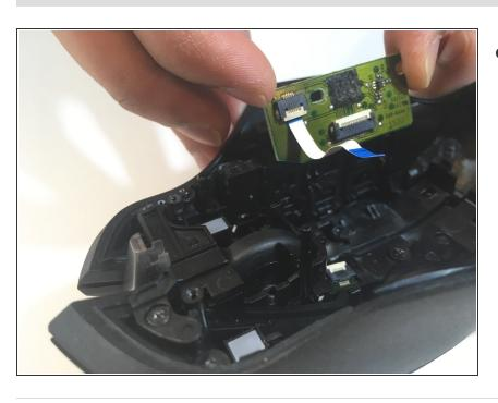
Use a black spudger and your fingers to loosen and remove the side motherboard.
