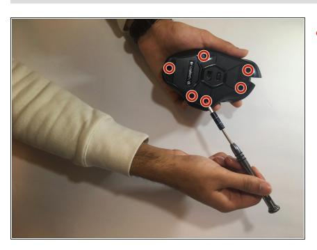
Use a Phillips #00 screwdriver to unscrew all 6 screws (3x5mm) from underneath the mice feet.
