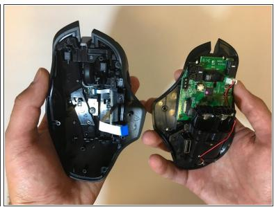
Use tweezers to grip and pull the white ribbon cable from the motherboard.
