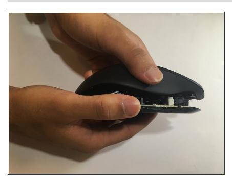
Lift the top of the mouse from the base of the mouse (separate the mouse in half) to expose the internal hardware.
