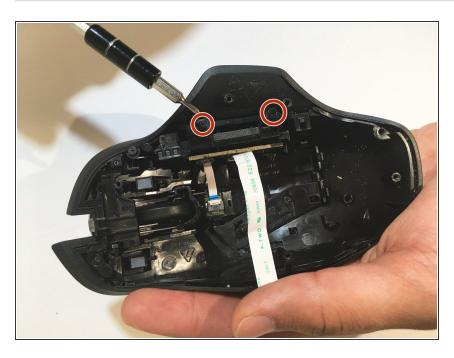
Use a Phillips #00 screwdriver to remove both screws (3x5mm) from above the side motherboard.
