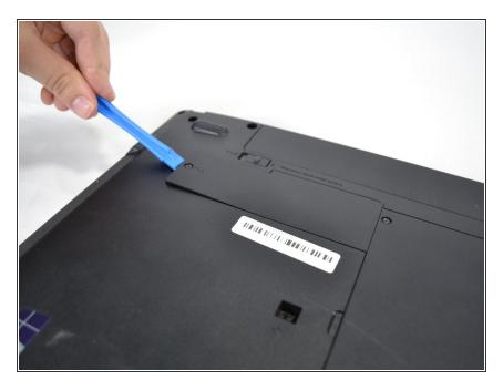
Use a plastic opening tool to remove panel.
