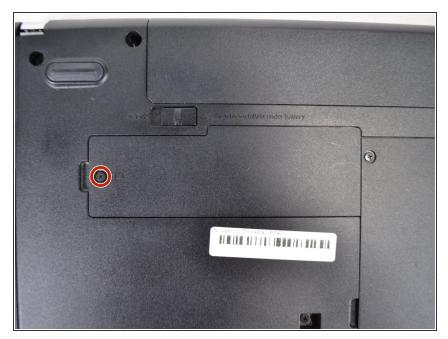
Remove the single 1mm Phillips #0 screw holding the small plastic panel in place.
