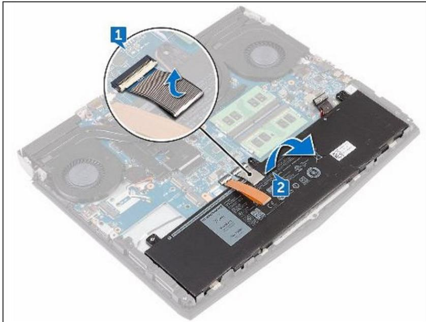
**⚠ CAUTION:** Ensure the keyboard and keyboard-backlit cables are not under the battery.
