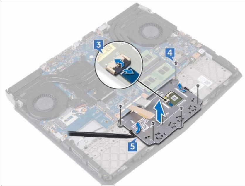
**⚠ CAUTION:** Ensure the keyboard and keyboard-backlit cables are not under the touch pad.
