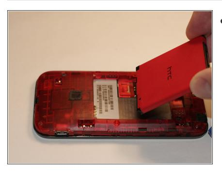
Remove the red battery to replace.
