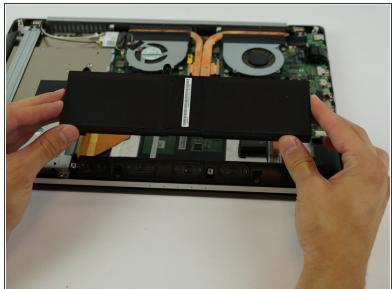
Using both hands, lift the battery vertically out of the device.
