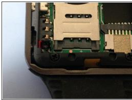
Next we need to remove the 4 screws in the corners, These can be removed with a 00 head
