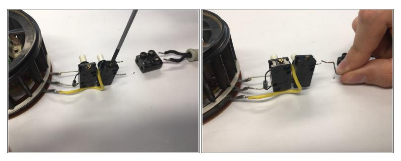
Loosen the flathead screws and remove the wires from the button holder. Remove the button holders. When you unscrew the wire opposite to where the yellow wire is connected, you can slide the button off of the middle wire connected to the motor.
