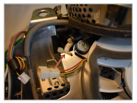
There may be a zip tie holding another cable to the fan assembly, cut it to remove the fan assembly.
