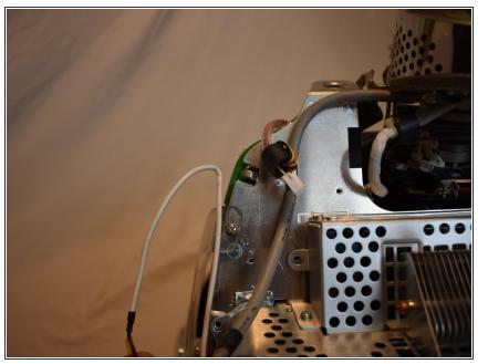
• The power button cable may be tucked in the casing, you will need to un-tuck it.
