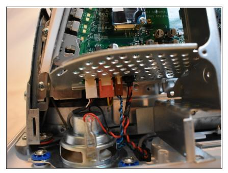
• There are four connectors at the bottom of the motherboard that must be removed.
