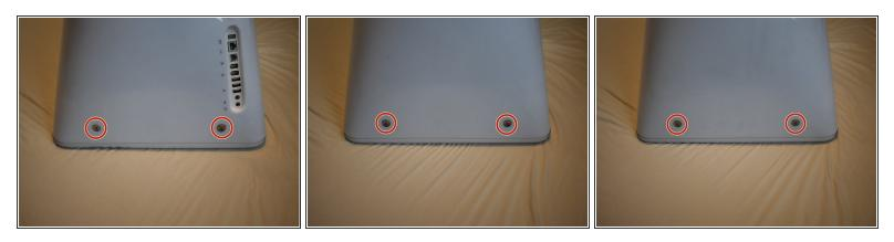
• Remove two 2.5mm hex screws from each of the other sides of the computer.
