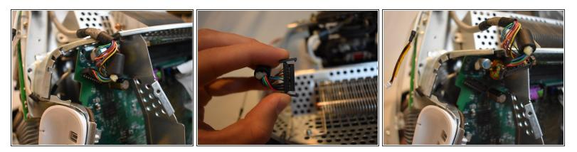
• There is a large display connector that must be removed. This can be done by squeezing the tabs and pulling.
