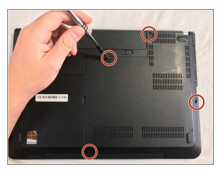
• Remove the four 2mm Phillips #00 screws from the bottom panel.
