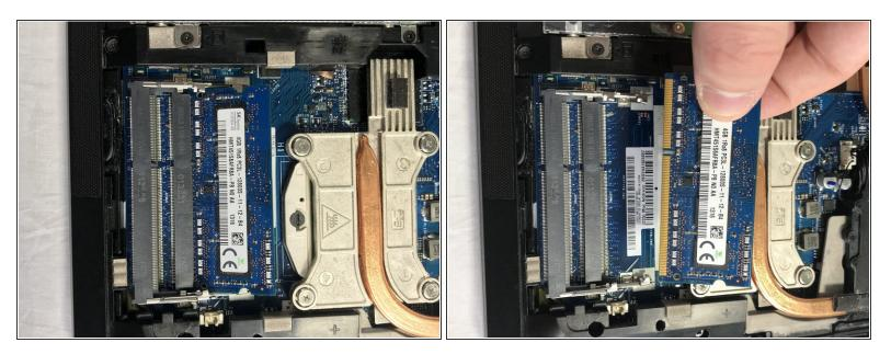
• Pull the RAM out at a 30 degree angle.
