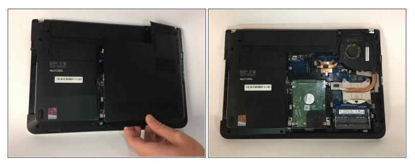
• Remove the back panel of the device.
