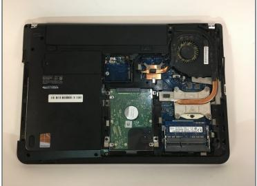
Remove the back panel of the device.
