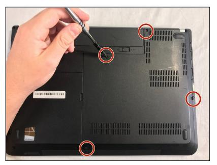
Remove the four 2mm Phillips #00 screws from the bottom panel.
