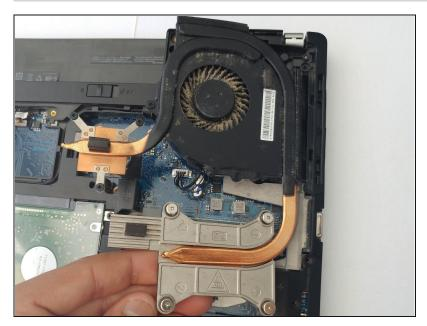
• Lift the fan assembly out of the laptop.
