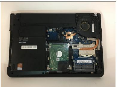
Remove the back panel of the device.
