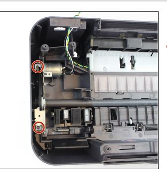
Remove the two 13mm screws which hold the paper roller motor frame in place.
