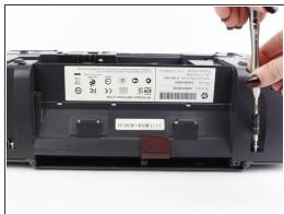
Remove the two 13 mm screws located on the back of the printer using a screwdriver with the T10 torx bit (star-shaped).
