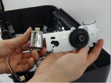
• Remove the remaining 4mm screw from the motor, then take the motor out.
