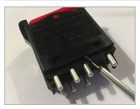
You must insert a blade or flat (thin) screwdriver into the existing slot in the base between the two small clasps, and gently pry
