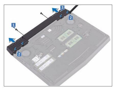
Remove the two screws (M2.5x6L) that secure the rear-I/O cover to the palm-rest assembly.
