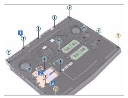
Remove the (M2x3) screw that secures the computer base to the palm-rest assembly.
