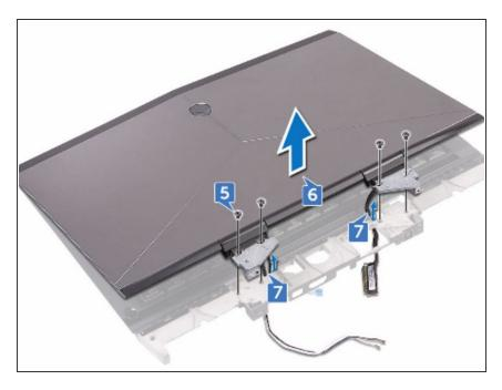
Align the screw holes on the display hinges with the screw holes on the palm- rest assembly.
