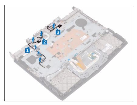
Route the logo-board cable through the routing guides on the palm-rest assembly.
