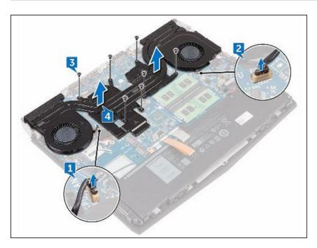
Disconnect the right-fan cable from the system board.
