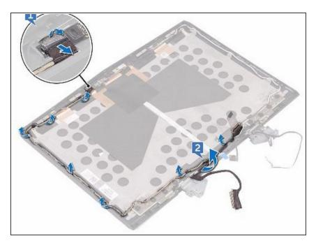
Note the camera cable routing and remove the cable from the routing guides on the display back-cover and antenna assembly.
