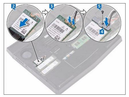
Align the screw hole on the wirelesscard bracket with the screw hole on the wireless card and the computer base.
