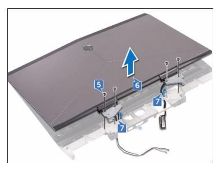
Lift the display assembly off the palm-rest assembly.
