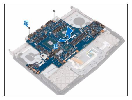
Replace the two screws (M2.5x6L) that secure the system-board to the palm- rest assembly.
