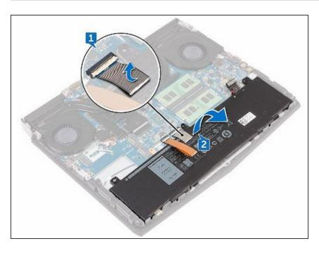
Lift the battery off the palm-rest assembly.
