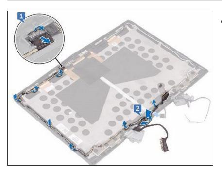
Connect the camera cable to the camera module.
