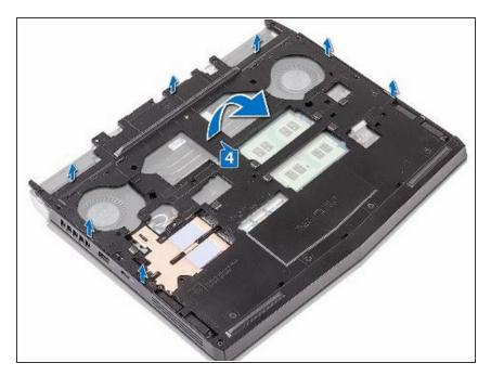
Remove the two (M2.5x6L) screws that secure the computer base to the palm-rest assembly.
