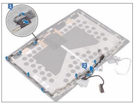
Route the **NEW** camera cable through the routing guides on the display back-cover and antenna assembly.
