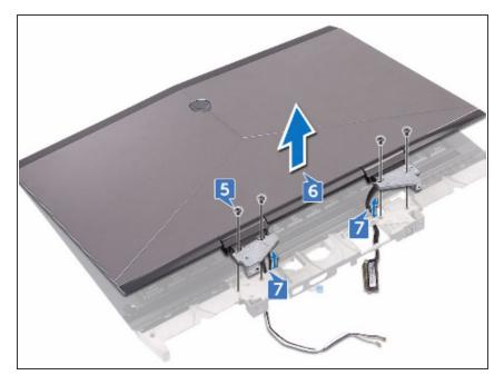
Replace the four screws (M2.5x6L) that secure the display assembly to the palm-rest assembly.
