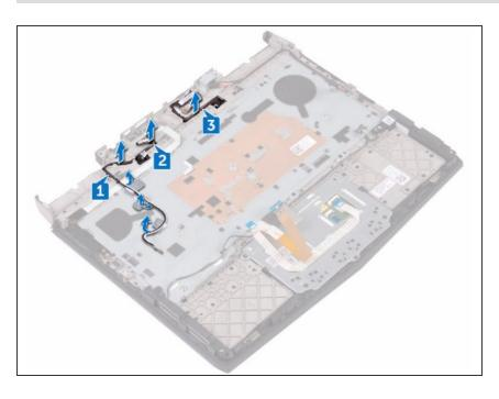
Remove the logo-board cable from the routing guides on the palm-rest assembly.
