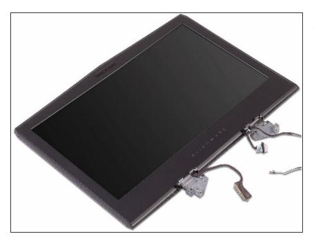
Route the cables through the routing holes on the palm-rest assembly.
