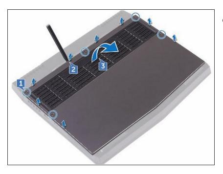
Tighten the five captive screws that secure the base cover to the computer base.
