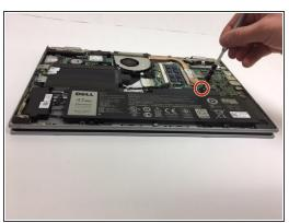
The battery will be the largest black component in the device located near the bottom edge. Using a Phillips #0 screwdriver, unscrew the two 3mm Phillips head screws holding in the battery.
