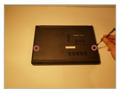
Use a J0 screwdriver to unscrew the two, 6mm Phillips screw on the rearcover.
