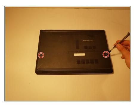
Flip the device on its back, locate the screws circled.
