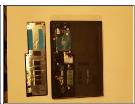
Using a spudger, Lightly lift the rear-cover up and at an angle, away from the computer.
