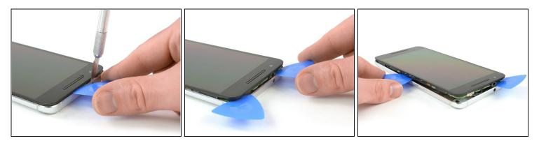
• Insert a razor knife between the metal back cover and the front glass to create a gap. Insert an opening pick into the gap and slide it to the top right corner.
