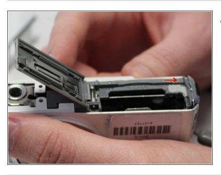
Slide the battery lock to the right and remove battery.
