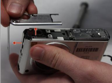
• Remove the remaining 3 mm screw holding on the side panel and remove the panel entirely.
