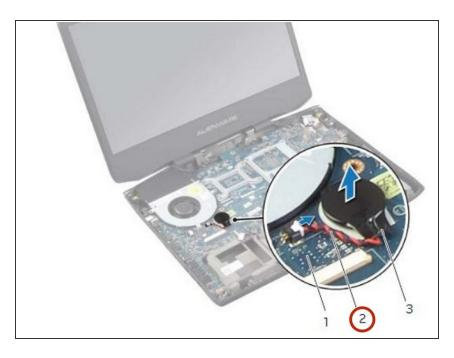
Lift the coin-cell battery along with its cable off the system board.
