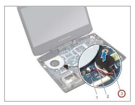
Peel the coin-cell battery off the system board.
