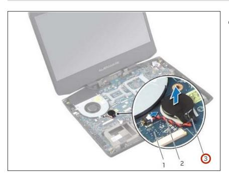
Connect the coin-cell battery cable to the system-board connector.
