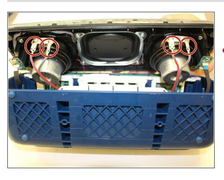
Once you have gotten to the internal parts of the speaker, there are seven wires connecting the speaker plate to the body of the speaker. Pinch the release tabs at the top of each of the four main wires to remove them.
