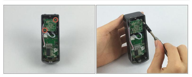
• Using the JIS #0 screwdriver, remove the 1mm screws from behind the camera.
