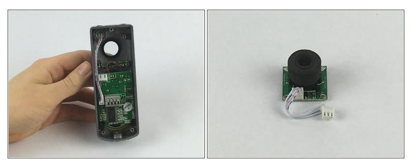
• Remove the camera from the device.
