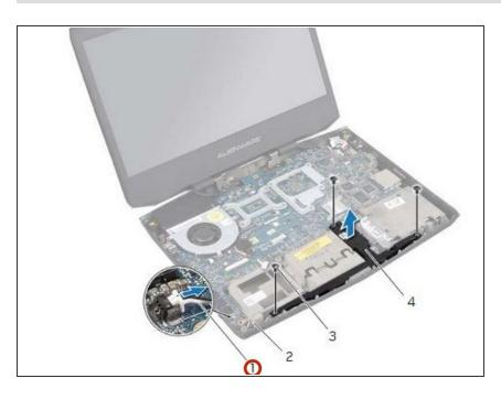
Note the subwoofer cable routing and remove it from the routing guide.
