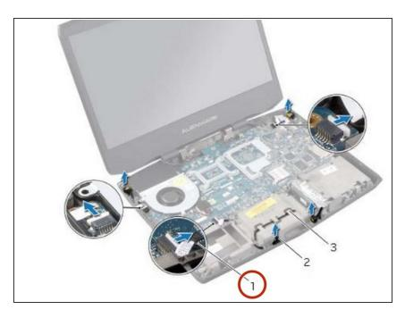
Connect the tron-light cables to their respective connectors on the system-board.
