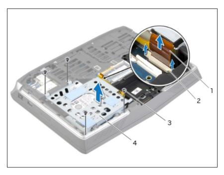
Align the screw holes on the secondary hard-drive with the screw holes on the secondary hard-drive bracket.
