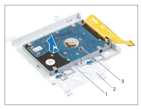
Place the **NEW** secondary harddrive in the secondary hard-drive bracket.
