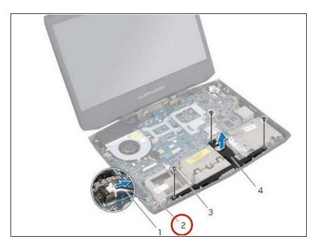
Lift the subwoofer along with its cable away from the computer base.
