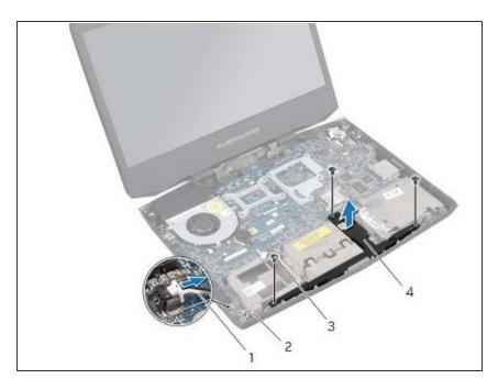
Use the alignment posts on the computer base to keep the NEW subwoofer in place.
