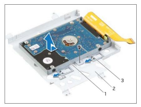
Replace the screw that secures the secondary hard-drive assembly to the main bracket.
