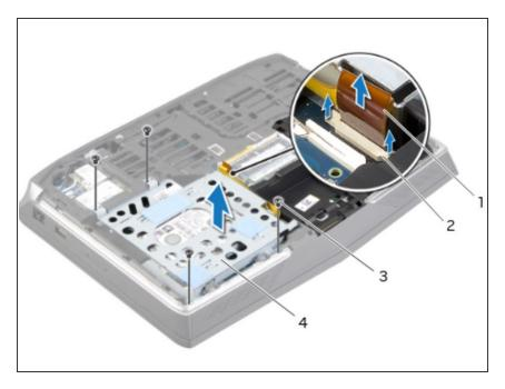
Turn the secondary hard-drive assembly over.
