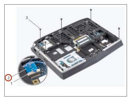
Slide the status-light board cable into the system-board connector and press on the connector latch to secure the cable.
