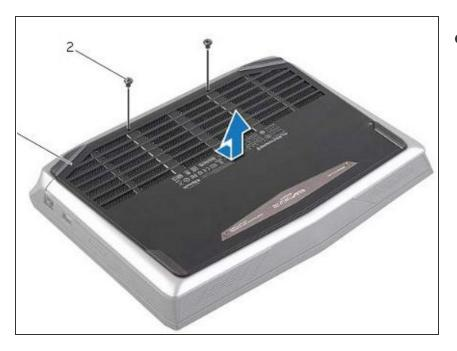
Replace the screws that secure the base cover to the computer base.
