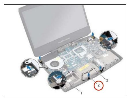
Connect the **NEW** tron lights to the optical fibres.
