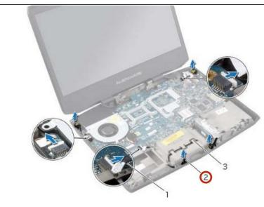
Route the tron-light cables through the routing guides on the computer base.
