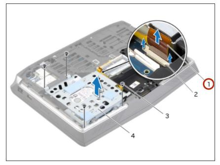
Slide the secondary hard-drive cable into the system-board connector and press down on the connector latches to secure the cable.
