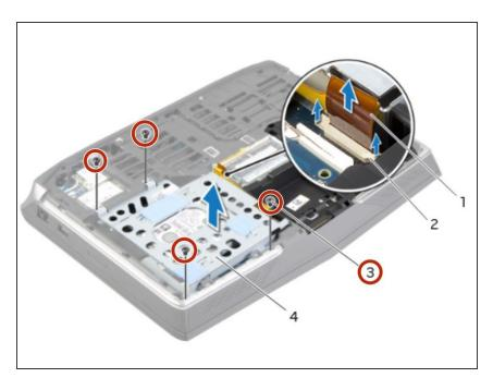
Align the screw holes on the secondary hard-drive assembly with the screw holes on the computer base.
