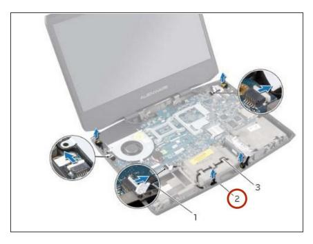
Disconnect the tron lights from the optical fibers.
