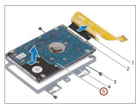
Connect the interposer to the secondary hard-drive connector.
