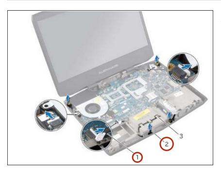
Lift the tron lights along with their cables off the computer base.
