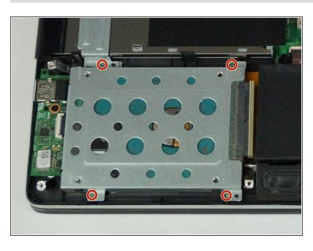
Remove the four 4mm silver Phillips #1 screws that are holding the hard drive in place.
