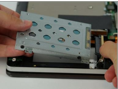
Lift up and remove the hard drive from the motherboard.
