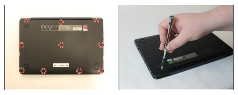
• Remove the back 6mm and 8mm screws with a J000 screwdriver.
