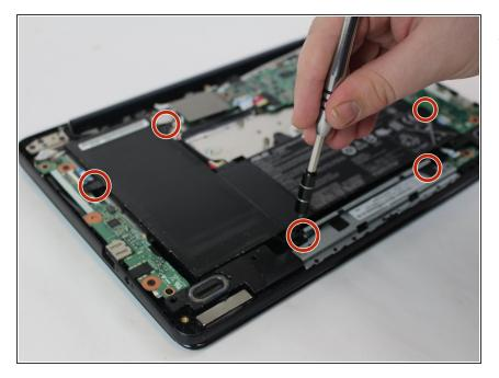
Unscrew the battery from the motherboard using a J000 screwdriver on the 3mm screws.
