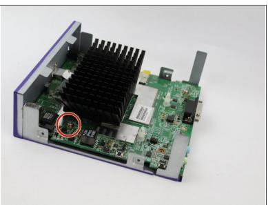
Remove the four 8mm screws at each corner of the motherboard with a JIS #0 screwdriver.
