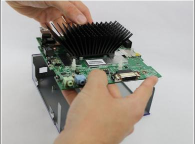
Lift the motherboard out of the casing.
