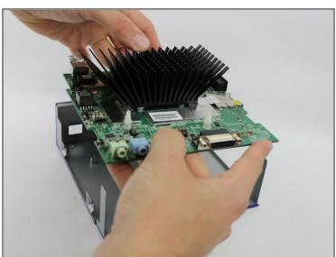
• Lift the motherboard out of the casing.
