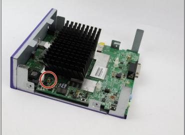
• Remove the four 8mm screws at each corner of the motherboard with a JIS #0 screwdriver.
