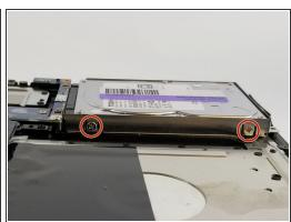
Use the Phillips head screw driver to remove four 4mm screws located on both sides of the hard drive.
