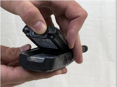
Push in the release button and pull up on the battery to remove.
