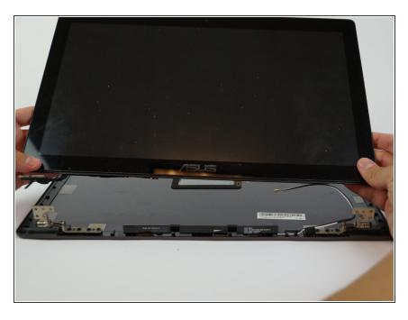
Lift the screen from the display to remove.
