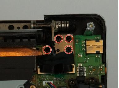
Remove the eight black 4mm Phillips #1 screws holding display to laptop base.
