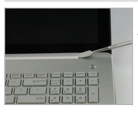
After removing the display from the board, slide the grey hinge cap to remove.
