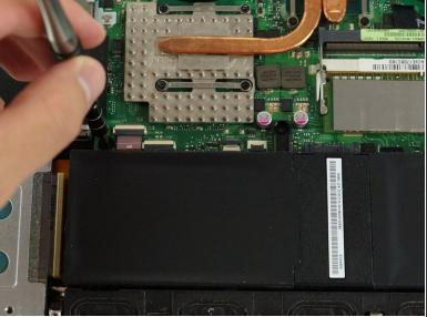
Remove the three 4mm JIS #0 screws from the battery.
