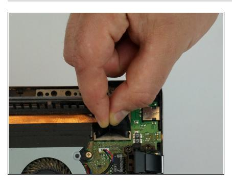
Lift the tab on the thick black wire to disconnect the display connector.
