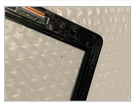
• Before installing new screen, ensure that the adhesive strips are laying flat around the edges, and clean the surface of the screen of debris from prying the old screen off. These will show up on the new screen if you sandwich them in between the glass and the screen. To reassemble your device, follow these instructions in reverse order.
