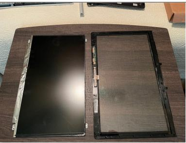
• Using a spudger or soft pry tool, work your way around the edge of the screen to separate the screen from the bezel adhesive strips. Take your time, and be careful not to break the bezel.
