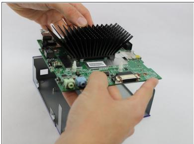
Lift the motherboard out of the casing.
