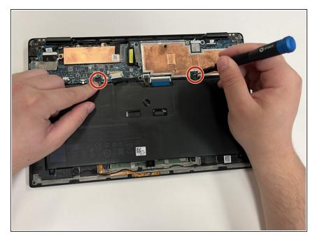
Use a Phillips #000 screwdriver to remove the two screws (M1.6x4) that secure the battery to the palmrest assembly.
