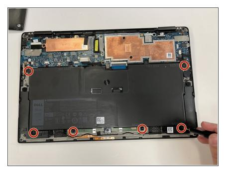
Use a Phillips #000 screwdriver to remove the six screws (M2x3) that secure the battery to the palm-rest assembly.
