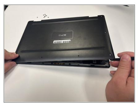
Starting from the front corner of the computer, pry up the base cover using a spudger and lift the base cover off the palm-rest assembly.
