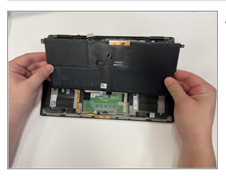
Lift the battery off the palm-rest assembly.
