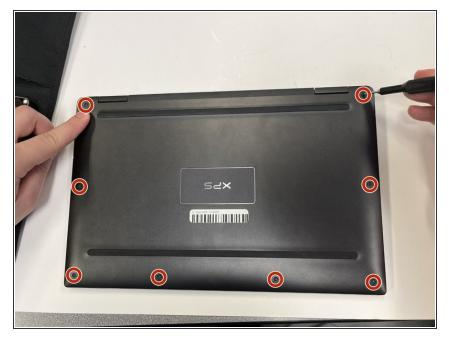
Use a Torx T4 screwdriver to remove the eight screws (M2x3) that secure the base cover to the palmrest assembly.
