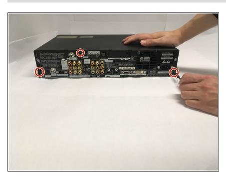
Remove the three 6.5 mm Phillips screws on the back of the device casing.
