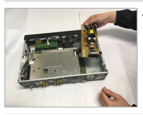
Remove the power supply board by pulling it toward the interior of the device then lifting.
