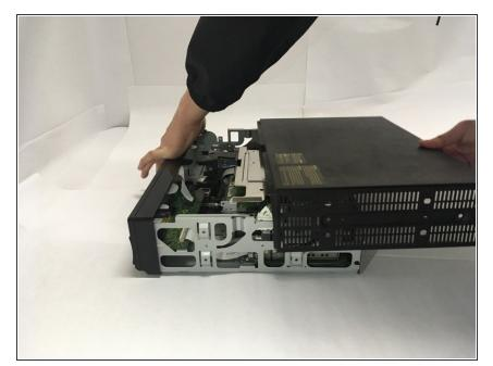
Grip the front panel in one hand and the back of the casing in the other.
