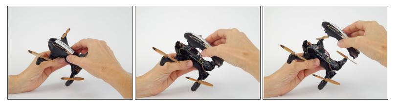
• Flip the drone over and lift off the top plastic shell of the drone.
