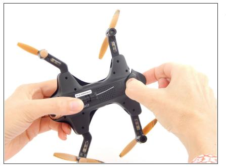
Grasp the tail end of the drone where the lip of the battery protrudes.
