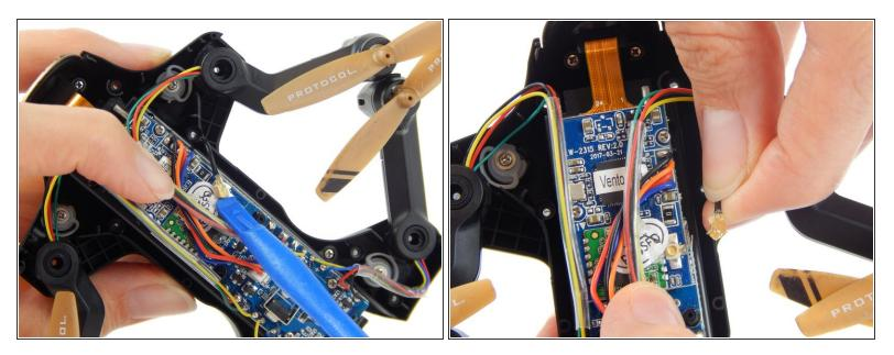
Pry the gold Wi-Fi antenna connector, located under the previously removed foam pad, away from the Wi-Fi transmitter board to disconnect it.
