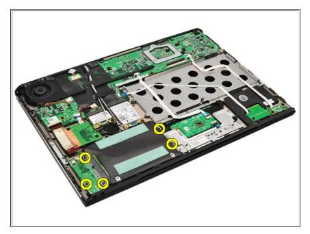
Remove the screws that secure the audio board and the hard drive to the computer.
