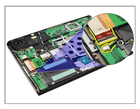
Disconnect the speaker and system board cables from the audio board.
