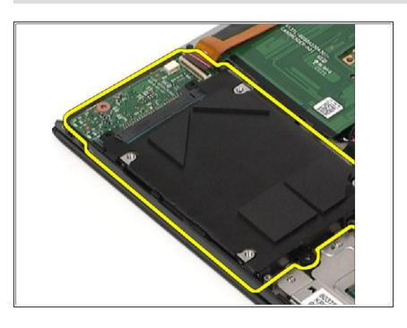
Lift and remove the hard drive and audio board assembly from the computer.
