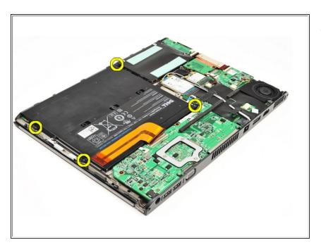
Remove the screws that secure the battery to the computer.
